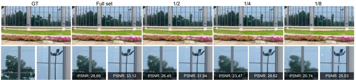
Fig. 10. **Varying the baseline of captured views.** In *Natatorium*, while quality stays reasonable with half the views, sharpness decreases with one quarter of the views as the camera baseline increases. At one eighth of the views, artifacts in thin features appear. PSNR metrics are reported for zoom-ins.
