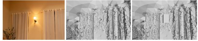
Fig. 20. *Left*: Captured input image of a light. *Middle*: Original geometry of the light obtained from the RealityCapture software. *Right*: Added proxy for the light that is later turned into a volumetric reconstruction.
