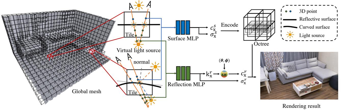
Fig. 2. *Scalable neural scene representation*. Tiles are allocated based on a global mesh proxy. Each tile has two MLPs: 1) The *surface MLP* that encodes density and view independent color, which is later stored in an octree for fast rendering. 2) The *reflection MLP* that encodes view-dependent effects like highlights using virtual points ‘underneath’ the surface at the ray distance of the reflected light. Color outputs from both paths are combined in the final rendering.
